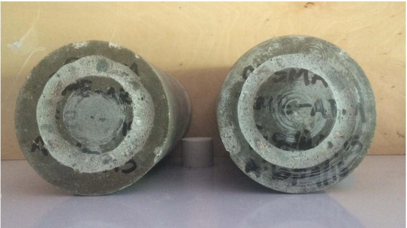
Figure 3: Photograph of test cylinders after abrasion testing- EdenCrete™ cylinder on the right with the shallower wear ring and far less visible aggregate
