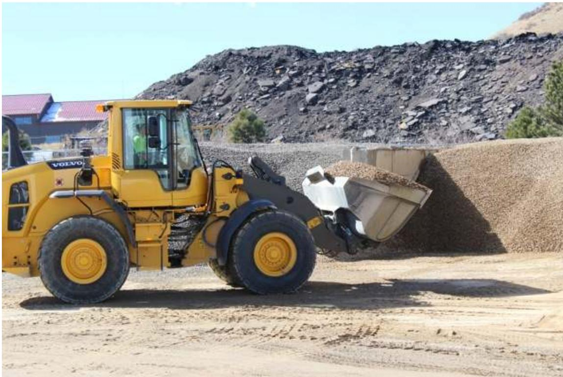
**Figure 3 Loader taking aggregate from existing aggregate bin**
