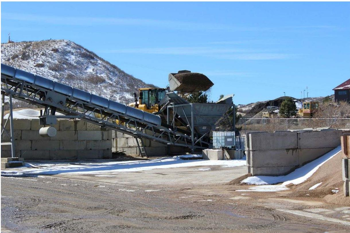
**Figure 2 Loading aggregate into hopper from aggregate bin**
