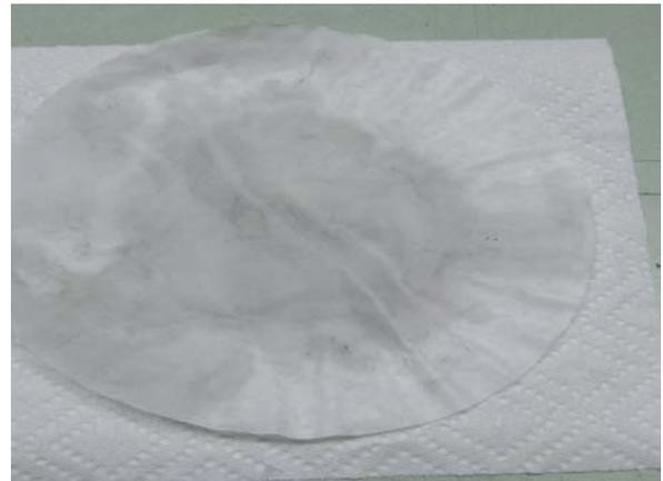
**Filter showing Very Little Trapped Carbon Using New Mixing Method**
