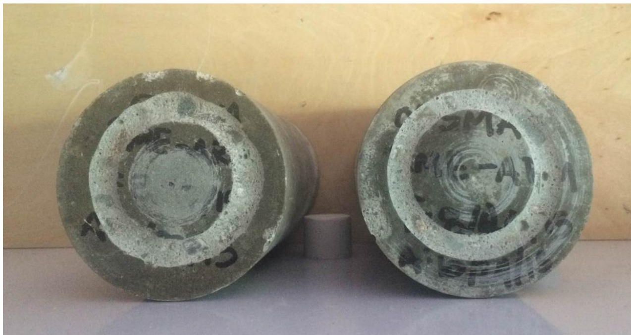
Figure 3: Photograph of test cylinders after abrasion testing- EdenCrete™ cylinder on the right with the shallower wear ring and far less visible aggregate
