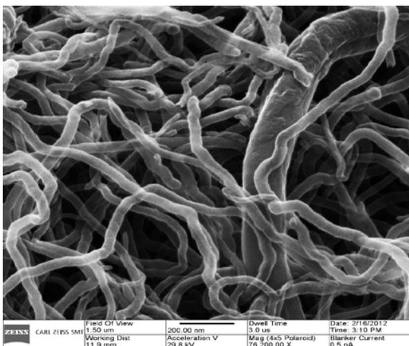
**Helium Ion Microscope Image of Eden's Carbon Nanotubes in Fresh Cement Paste** (showing build-up of dense hydrated cement on the surface of the CNT (top right) due to CNT acting as nucleating points for cement hydration)
