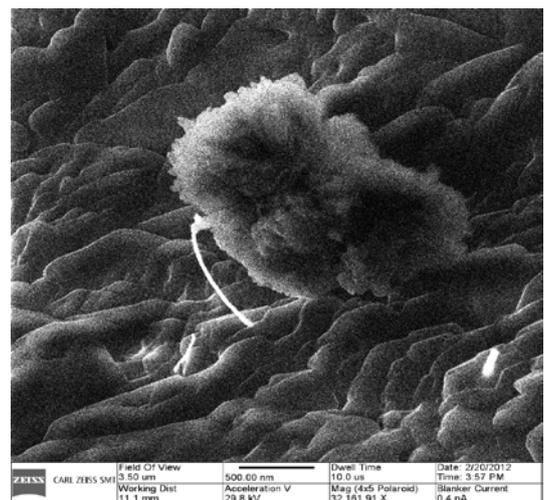
**Helium Ion Microscope Image of Eden's Carbon Nanotubes in Hardened Cement Paste after Fracturing** (showing that the ends of the CNT are well-bonded within the cement gel and provide anchorage)
