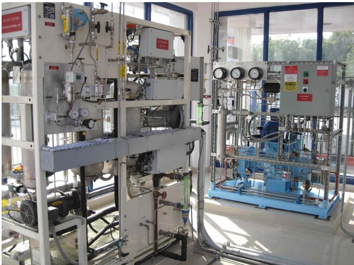
Figure 2 The electrolyser and compressor at the Dwarka Hythane® Station
